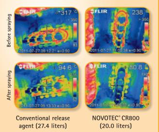
Left: Casting process with 1:100 wax free dye lubricant. Right: Casting process with 1:800 diluted NOVOTEC\* CR800 but 30% less sprayed water.
